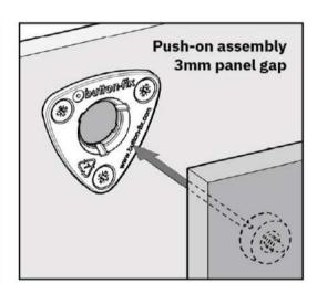
The Type 3 Fix can be surface-mounted, creating an 8mm gap between the panels, or semi-rebated to reduce the gap to 3mm. Align the Buttons with the Fixes and press firmly until each Button-fix goes 'click'. No clearance at the sides of the panel is required for assembly or removal.
