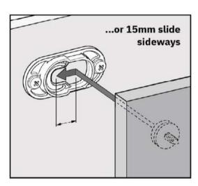
The Type 1 Metal Fix can be surface-mounted, creating an 8mm gap between the panels, or semi-rebated to reduce the gap to 3mm. Engage the Buttons in the Fix and slide the panel down by 15mm, until Button-fix goes 'click'. The Type 1 Metal Button-fix can be configured for sideways assembly too.
