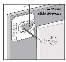
The Type 1 Bonded Fix can be surface-mounted, creating an 8mm gap between the panels, or semi-rebated to reduce the gap to approximately 2mm. Engage the Buttons in the Fix and slide the panel down by 15mm, until Button-fix goes 'click'. The Type 1 Bonded Button-fix can be configured for sideways assembly too.
